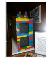
The first Google computer at Stanford was housed in custom-made enclosures constructed from LEGO bricks.
