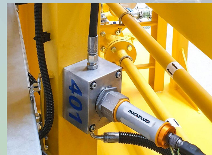
In-line breakdown voltage measurement with MicaSonic™
