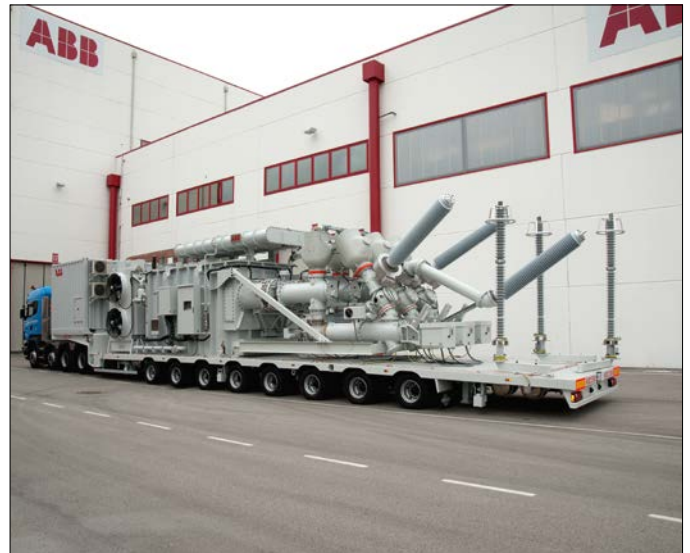
Figure 6. Power transformers for mobile substations can be easily arranged in many configurations, mounted for air, rail and road transportation and installed almost anywhere.
