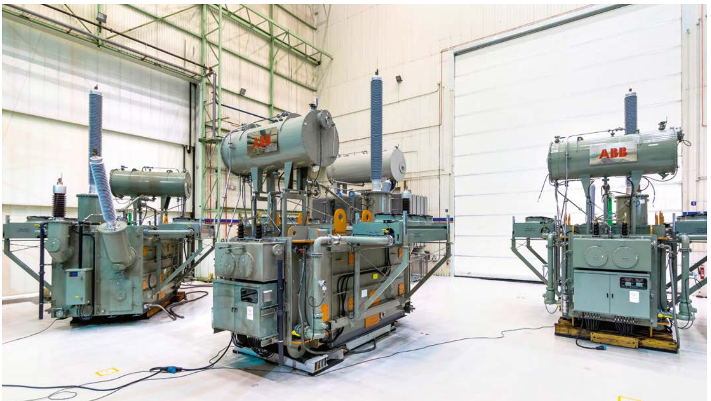
Figure 4. Polytransformers rely on a multi-voltage approach and are compact; they can be shipped and installed in any substation.
