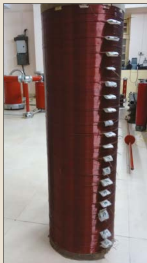
Figure 1a. Single-layer winding
