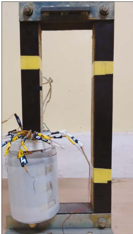
Figure 4a. 10 section multi-layer winding
