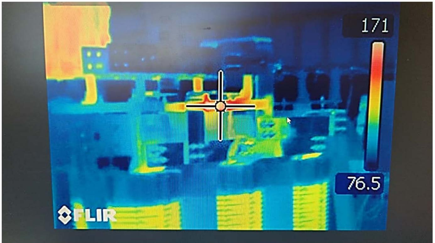
Figure 2. Infrared camera image of the temperature distribution in the magnetic busbar support
