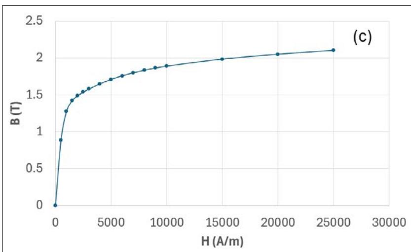
Figure 3. a) 3-D simplified transformer model, b) busbar support model, c) magnetization curve for mild steel
